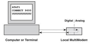
Figure C-1. Local analog loopback test.
